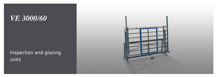
Inspection and glazing unit for glazing and final inspection. Quick and precise assembly of windows, doors and elements. Stable steel construction. Precision ensured through parallel clamping bar pressing technique with manually operated pressing bars. Easy operation by means of foot switch. Pneumatic centring, storage area for tools and 4-fold compressed air supply.
