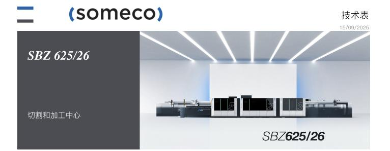
Automated CNC through-bar machining line consisting of specific units for milling, drilling, V-notch, cutting, contouring and fastening reinforcements. The line is designed for high capacity production.
