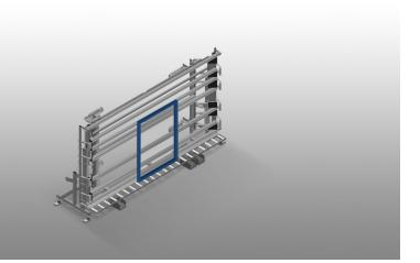
Inspection and glazing unit for glazing and final inspection in individual and serial assembly line production. Quick and precise assembly of windows, doors and elements. Stable steel construction. Precision ensured through parallel clamping bar pressing technique. Height continuously adjustable. Easy operation by means of foot switch. Two pressing bars which fold down and can be moved pneumatically and 4-fold compressed air supply.
