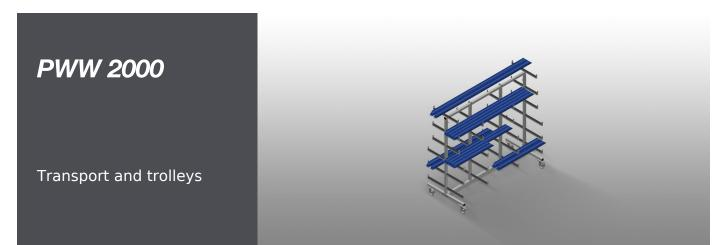
Profile trolley for horizontal storage and transportation of profiles. Stable steel construction. Horizontal profile transportation. Support arms are rubber coated. Profile trolley with profile supports on both sides. Six supports per upright. Two centre uprights. Four castors, two of which have a fixing brake. Option: individual centre upright.
