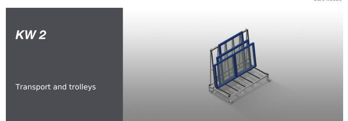
Commissioning trolley for in-house and truck transportation of window elements. Stable steel construction. Trolley for in-house and external transportation. Openings for forklift transportation. Four hooks for crane transportation. Four lashing strap attachment points. Profile supports with rubber surface. Castors can be removed for increased stability of the commissioning trolley in a lorry. Four castors, two of which have a fixing brake.
