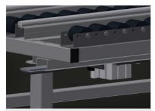
Pneumatic lifting unit (Optional) Lifting unit L = 3.000 mm
