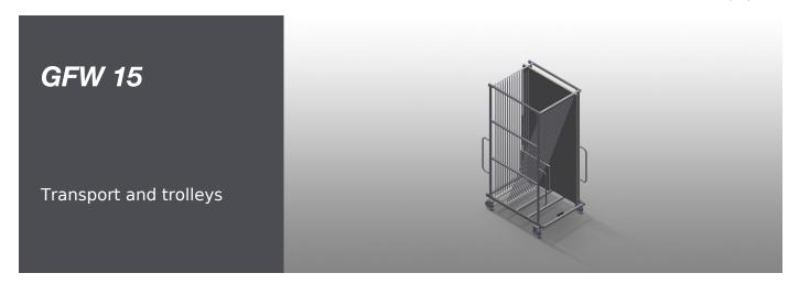
Stable steel construction. Glass sorting. For in-house transportation of sheets of glass. Compartment dividers for 15 sheets of glass. Access is possible from both sides. The glass supporting surface has a rubber profile. Compartment divider with plastic protector. Transport handle on both sides for mobility. Two castors and two fixed rollers.
