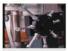
8-fold height adjustment (Optional) 8-fold height adjustment for different screw driving heights
