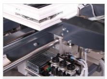
Screwing unit Mobile screwing unit with pneumatic height adjustment
