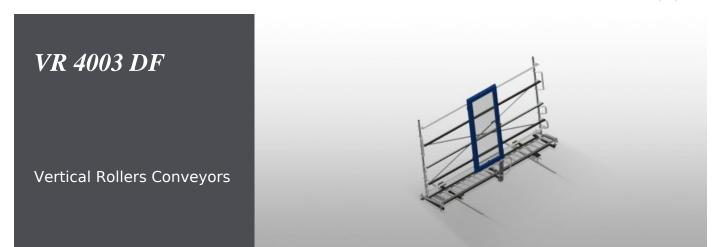
Stable steel construction. Vertical roller conveyor for smooth transportation to the next work task as well as for transportation to storage and sorting of the finished windows. Easy handling of window elements. Every roller conveyor unit is 4.000 mm long. Plastic slide bars top and bottom. Three mini-roller conveyors with rubber rollers, diameter 50 mm. Basic unit with end rack. Vertical roller conveyor on rails with flanged rollers, mobile. Roller conveyor can be rotated 360°.
