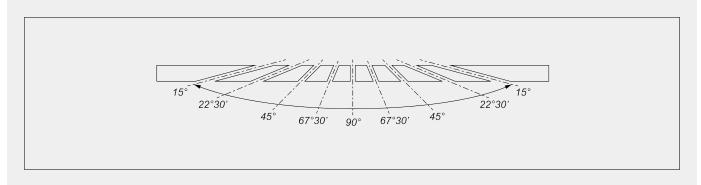
Mechanical adjustment of intermediate angles
