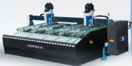
Automatic workbench for the automated screwing. Screwing operation process done simultaneously by two separate fully automatic screwing axis-controlled units. All machine axes are moved by hardened steel ball screw and rack-pinion gear system that provides accuracy and durability. The precision of positioning with 0,1 mm accuracy by high-speed servo on the holder axis. The machine is fully compatible with Processing center in automatic operation.
