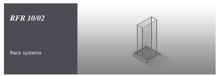
Rack for storage of frame elements. Stable steel construction. Rack for storage of frames. The individual elements are available for direct access. Specially designed for integration in assembly lines. Access is possible from both sides. Floor support equipped with knob profile. Compartment separating bars covered with protective tubing. Supporting surface with rollers for even easier loading and unloading.
