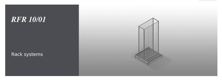
Rack for storage of frame elements. Stable steel construction. Rack for storage of frames. The individual elements are available for direct access. Specially designed for integration in assembly lines. Access is possible from both sides. Floor support equipped with knob profile. Compartment separating bars covered with protective tubing. Supporting surface with rollers for even easier loading and unloading.
