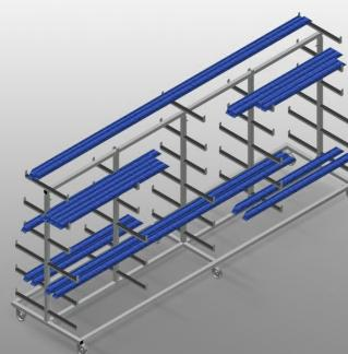
Profile trolley for horizontal storage and transportation of profiles. Stable steel construction. Horizontal profile transportation. Easy transportation of profile raw materials and cut-to-size profiles. Support arms are rubber coated. Profile trolley with profile supports on both sides. Six supports per upright. Three centre uprights. Six swivel castors, two of which with locking stop.
