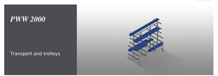
Profile trolley for horizontal storage and transportation of profiles. Stable steel construction. Horizontal profile transportation. Support arms are rubber coated. Profile trolley with profile supports on both sides. Six supports per upright. Two centre uprights. Four swivel castors, two of which with locking stop.
