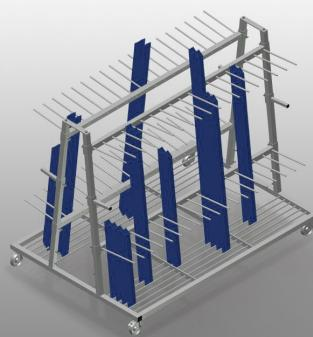
Profile trolley for vertical storage and transportation of profiles. Stable steel construction. Vertical profile transportation. Profile trolley can be loaded on both sides. 18 compartments per side. Easy loading and unloading. Sufficient for 120 - 160 profile bars. Compartment dividers height is adjustable. Supporting surface with bar grid floor. Four swivel castors, two of which with locking stop.
