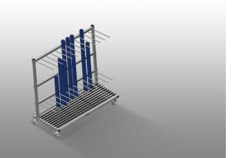
Profile trolley for vertical storage and transportation of aluminium profiles. Stable steel construction. Ideal for transportation and space-saving intermediate storage of cut-to-length profiles. Vertical profile transportation. Sufficient for 12 – 60 profile bars. Compartment divider height is adjustable. Lower supporting surface with rubber strips. Compartment dividers with protective tubing. Rear back support with rubber strips. Four swivel castors, two of which with locking stop.
