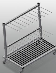
Profile trolley for vertical storage and transportation of aluminium profiles. Stable steel construction. Ideal for transportation and space-saving intermediate storage of cut-to-length profiles. Vertical profile transportation. Sufficient for 30 - 40 profile bars. Compartment divider height is adjustable. Lower supporting surface with rubber strips. Compartment dividers with protective tubing. Rear back support with rubber strips. Four swivel castors, two of which with locking stop.
