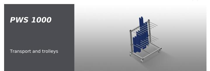
Profile trolley for vertical storage and transportation of profiles. Stable steel construction. Vertical profile transportation. Profile trolley with loading on one side. Easy loading and unloading. Sufficient for 30-40 profile bars. Compartment divider height is adjustable. Supporting surface with bar grid floor. Four swivel castors, two of which with locking stop.
