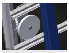
**Clamps** Two material clamps at the side fix the profile while working, profile clamping height, max. 200 mm
