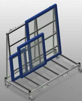
Commissioning trolley for in-house transportation of window elements. Stable steel construction. Trolley for in-house transportation. Openings for forklift transportation. Four hooks for crane transportation. Four lashing strap attachment points. Profile supports with rubber surface. Castors can be removed for increased stability of the commissioning trolley. Four swivel castors, two of which with locking stop.
