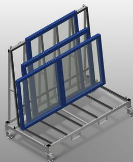
Commissioning trolley for in-house and truck transportation of window elements. Stable steel construction. Trolley for in-house and external transportation. Openings for forklift transportation. Four hooks for crane transportation. Four lashing strap attachment points. Profile supports with rubber surface. Castors can be removed for increased stability of the commissioning trolley in a lorry. Four swivel castors, two of which with locking stop.
