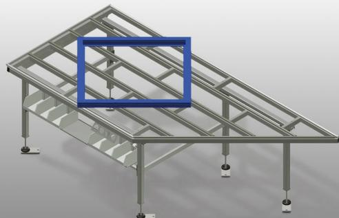
Horizontal table for all work tasks on frames and sashes. Stable steel construction. Angled work table; can be used as a pass-through in the production line or as a buffer zone. Assembly table for all work tasks on frames and sashes. Table supporting surface with plastic slide bars. Storage tray for setting down tools and accessories. Adjustable height. Simple installation with a modular system design.
