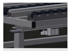
Pneumatic lifting unit (Optional) Lifting unit L = 1.000 mm
