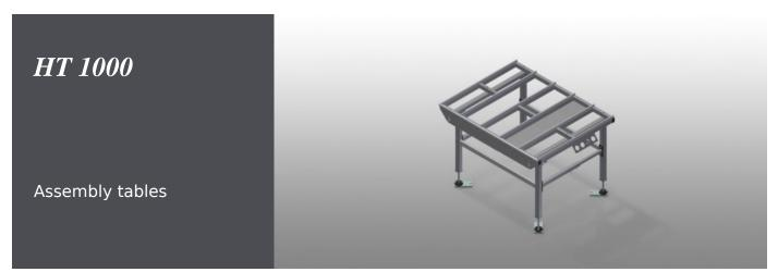
Horizontal table for all work tasks on frames and sashes. Stable steel construction. Table supporting surface with plastic slide bars. Storage tray for setting down tools and accessories. Adjustable height. Simple installation with a modular system design.
