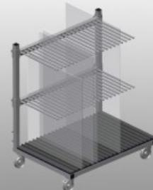
Glass transport trolley with sorting rack. Stable steel construction. Ideal for sorting glass. Hardwood supporting surface with felt. Compartment dividers for 20 sheets of glass. Compartment dividers height is adjustable. Four swivel castors, two of which with locking stop.
