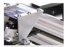
Laser unit (Optional) Laser for screw driving position
