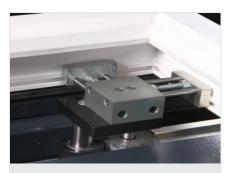
Stop block Two stop blocks for two sash widths
